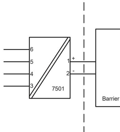
The barrier must not be connected to any associated apparatus which uses or generates more than 250 VRMS
